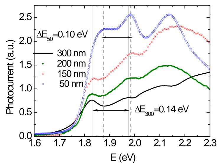
Photocurrent spectra of OTFTs with different active pentacene layer thickness  $\longrightarrow$  PC can monitor the gradual modification of the molecular packing.
