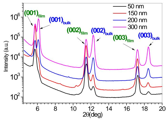
X-ray diffraction curves of pentacene thin films of different thickness  $\longrightarrow$  <u>Bulk phase dominates over 150nm</u>
