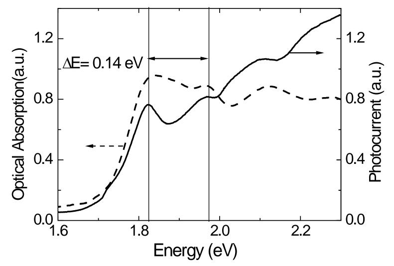
PC (solid line) and OA (dashed line) spectra of a pentacene thin film 300nm thick — Good agreement!
