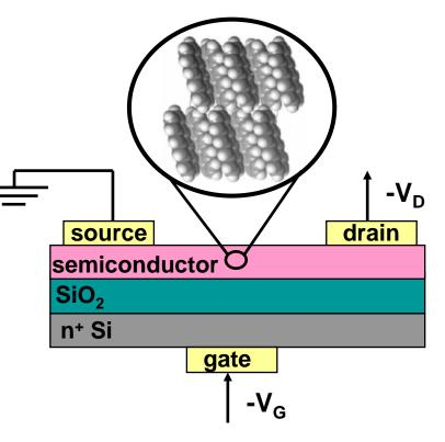
In OFET the conductivity is controlled by  $V_{GS}$ , only in the first layers of the SC (thin film phase) near the insulator interface.
