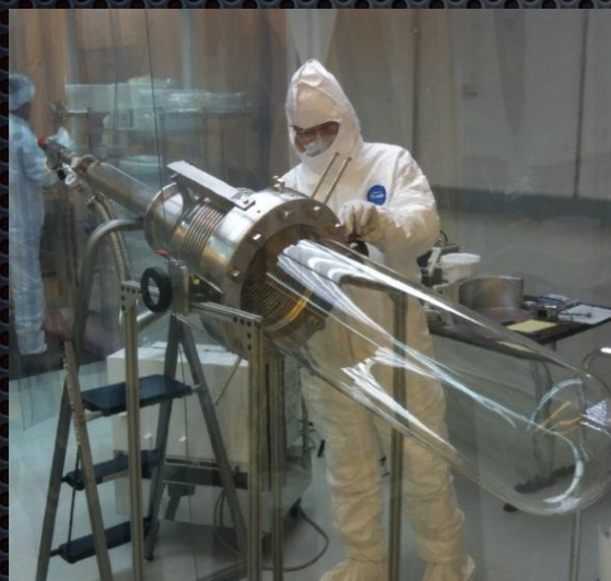
COUPP 60 kg CF_3I detector installed at SNOLAB; physics run until May 2014
