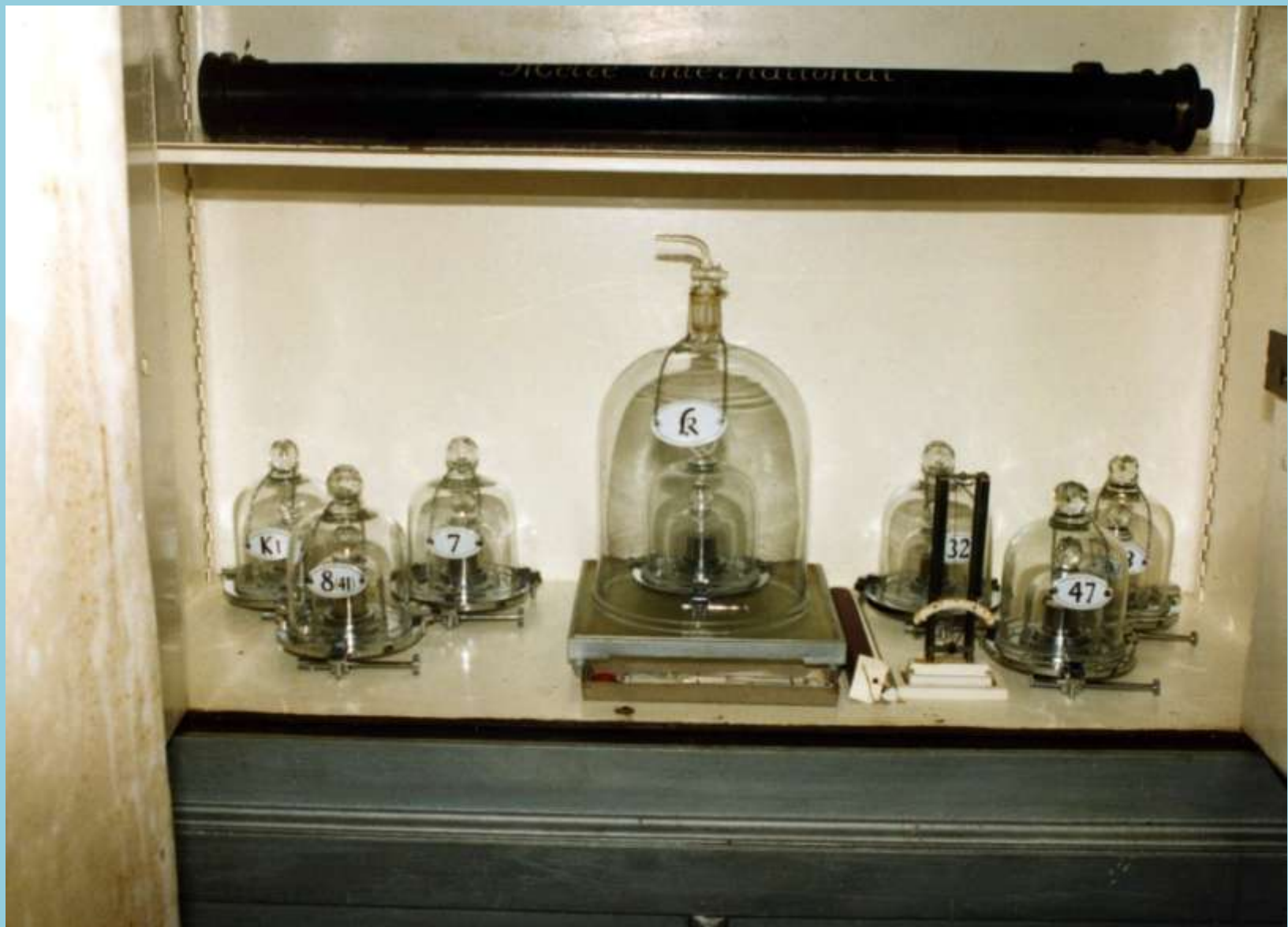
The vault of the prototypes containing the International prototypes of the metre and the Kilogram plus their official copies. This was replaced by a modern safe in the 1990s
