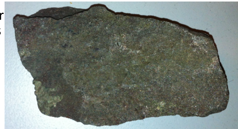
Monazite sample containing 2 to 3% of thorium mixed with rare earths (from the Steenkampskraal mine, South Africa – Trevor Blench)
