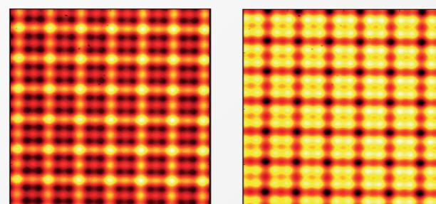
xy-lattice short lattice spacing 1.2 μm
