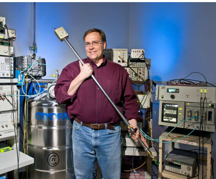
Sam Benz holding a 10 V PJVS probe
