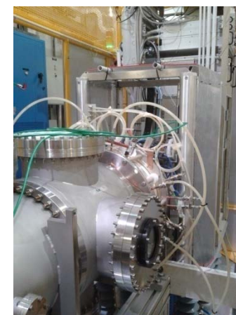
Some water cooling loops for extraction grid EG
