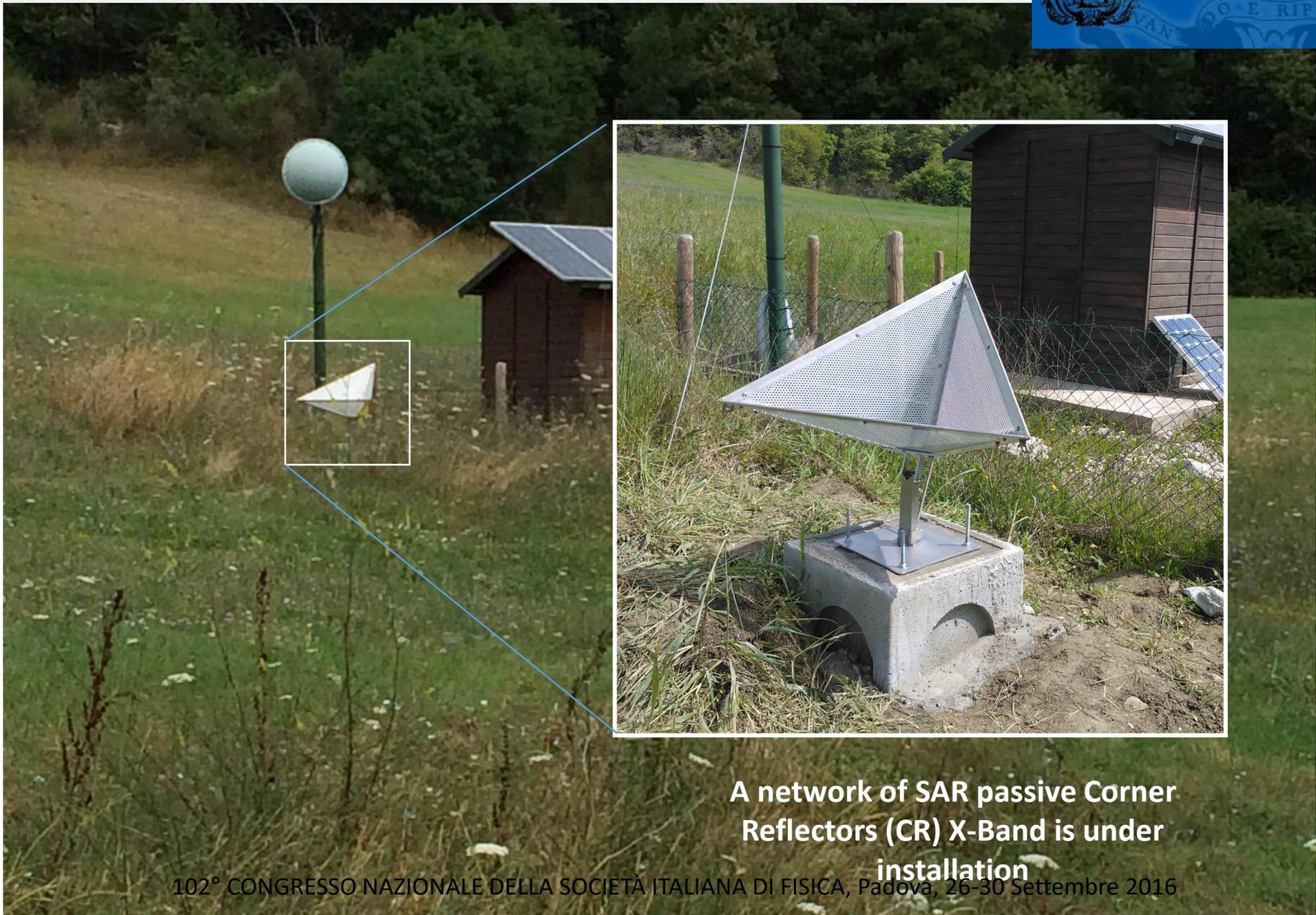
**A network of SAR passive Corner Reflectors (CR) X-Band is under installation**
