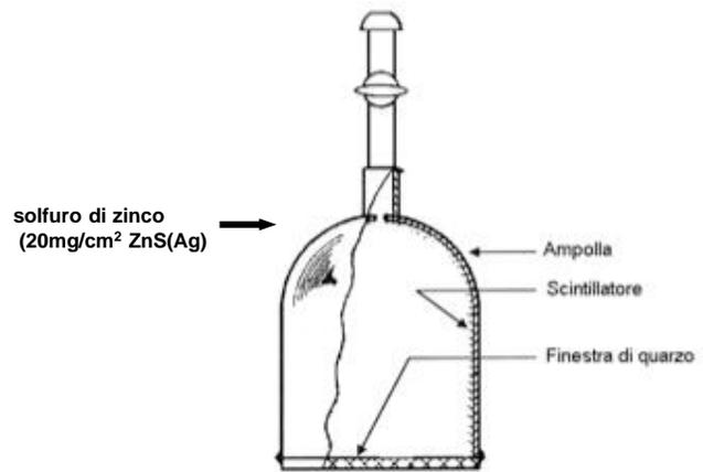
The detector is based on a Lucas cell powered by a 12V battery charged by a power supply connected to 220V or to a solar panel.
