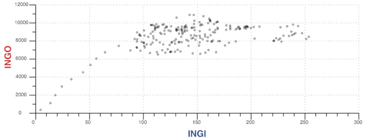
**Fig. 12** INGO radon concentration versus INGI radon concentration during the period from January 2015 to April 2015.
