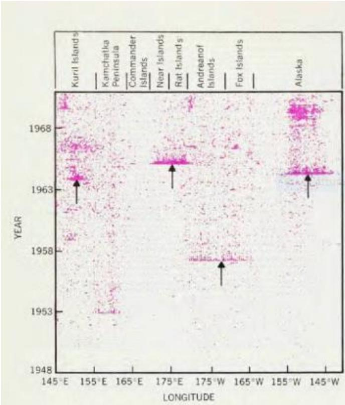
**Space-time plot** of earthquakes in northwest basin of the Pacific shows major events and aftershocks (arrows) preceded by gaps in seismic activity. The greater number of points in recent years reflects the improved density and quality of recording instruments. (Unpublished data from E. R. Engdahl.) Figure 2
