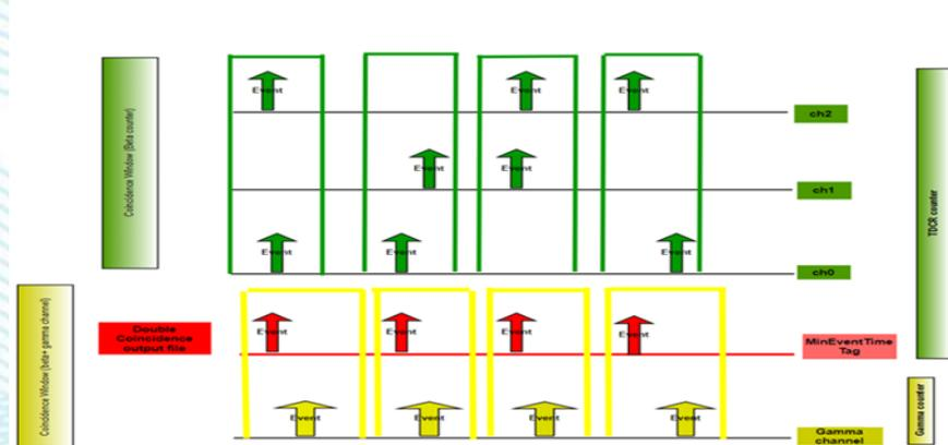
coincidence logic between gamma channel and double in TDCR counter (beta channel) with new coincidence window
