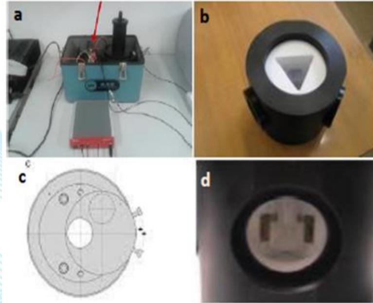
The portable TDCR system at ENEA. (b, d) The external and the internal view (up and down) respectively of the optical chamber(c) Optical shutter design.
