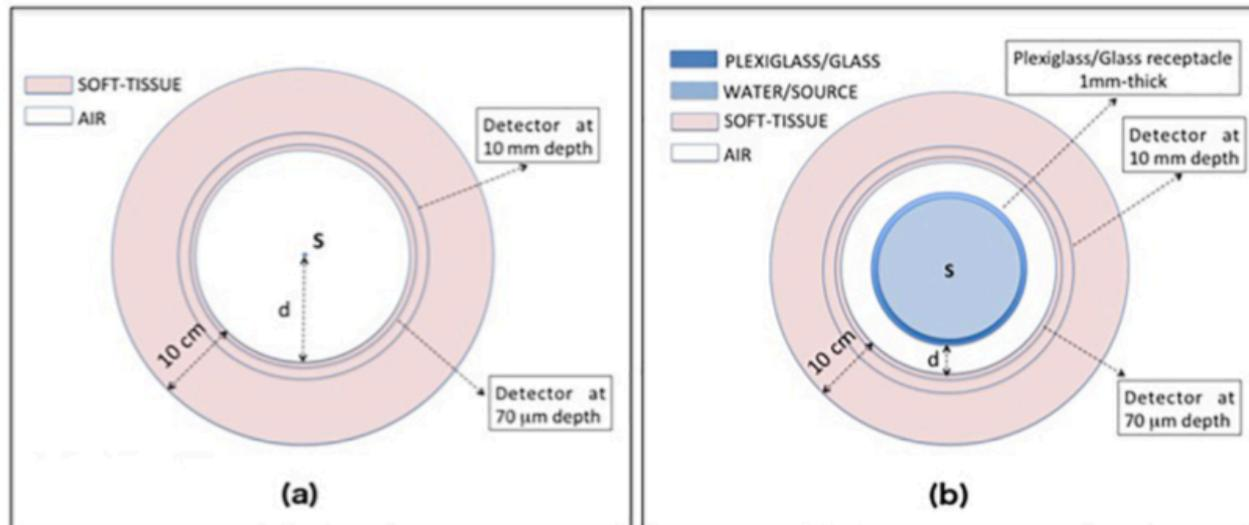
Fig. 3. Sketch of the adopted geometries: (a) Point-like source with  $d = 10, 30, 50, 100$  cm and (b) cylindrical source (both plexiglass and Pyrex glass vials) with  $d = 0, 10, 30, 50, 100$  cm.
