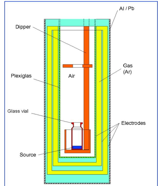
Figure 2. Schematic view of the Veenstra model VDC-405 dose calibrator.
