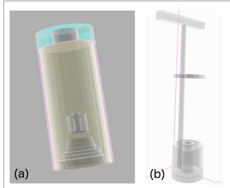
Figure 3: (a) 3D layout of the geometry reproduced in MC simulations; (b) detail of the vial holder inside the ionization chamber.
