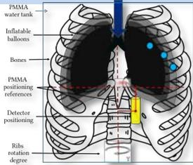
01 4D phantom with respiratory stop-motion and adjustable geometry for translational research
