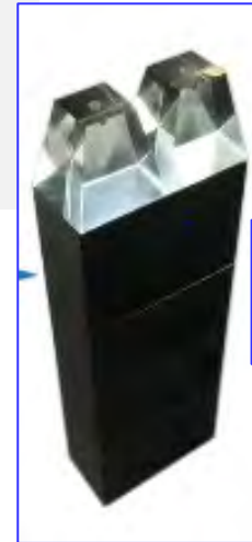
sPHENIX Wpowder/SciFi Cal Sensor: Si PMs
