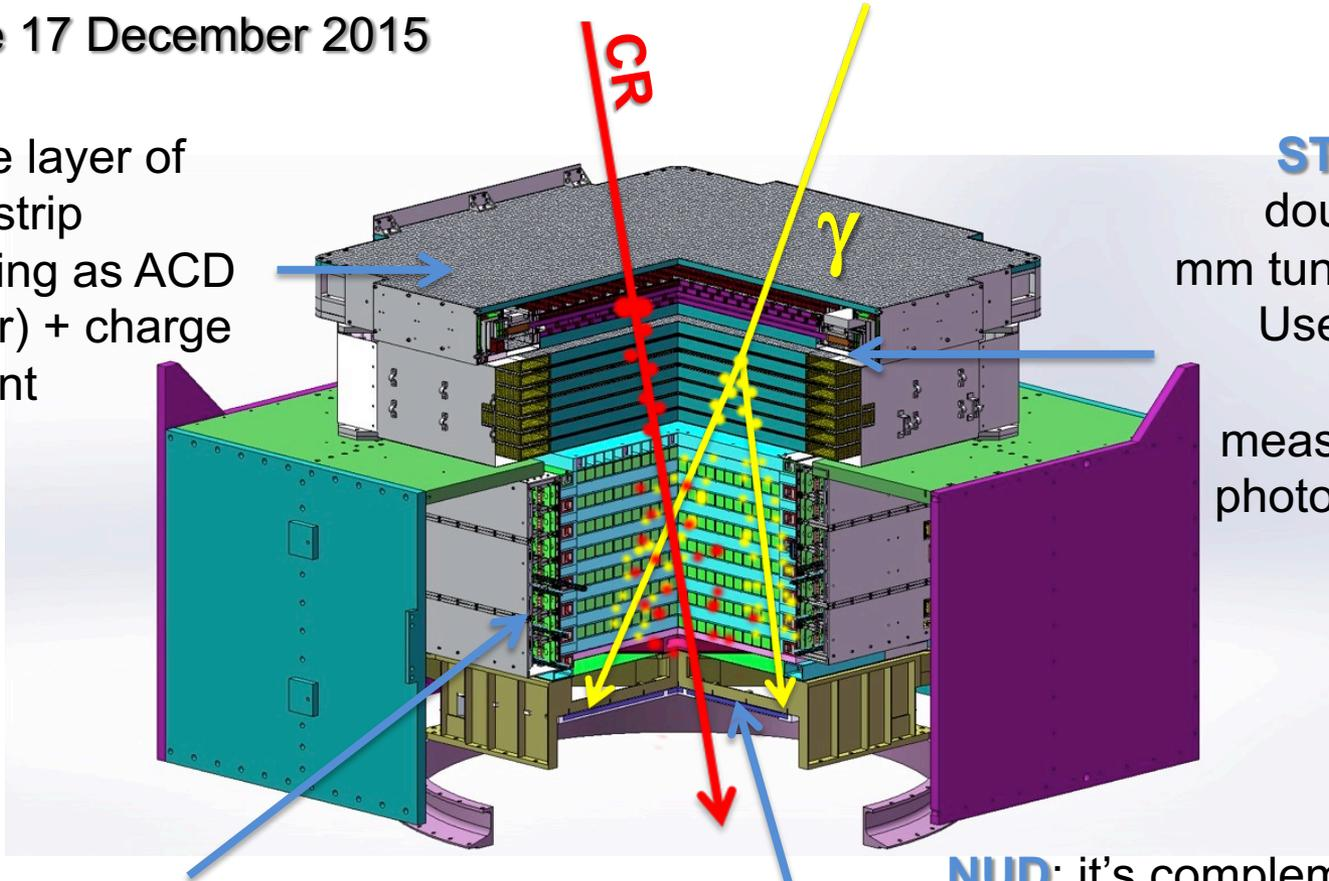
**STK:** 6 tracking double layer + 3 mm tungsten plates. Used for particle track, charge measurement and photon conversion ( $\sim 2 X_0$ )
