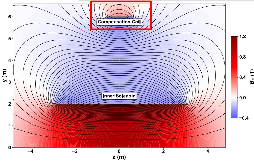
An (expandable) compensation coil balances the magnetic moment of the solenoid and allows the attitude control of the instrument within the heliospheric magnetic field
