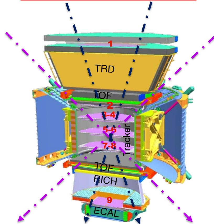
All the current and past detectors are designed as 'telescopes': they're sensitive only to particles impinging from "the top"
