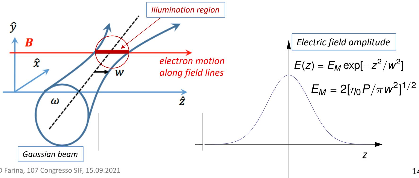
Nonlinear theory applies either to extremely high power sources or quite low energy particles as in the very early stage of a discharge (*D Farina, NF 2018*)
