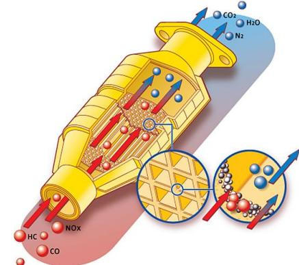
three-way catalytic converters
