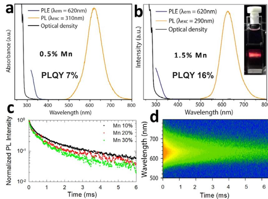
Orange emission due to  ${}^6\text{T}_1 \rightarrow {}^6\text{A}_1$  Transitions of  $\text{Mn}^{2+}$  dopants
