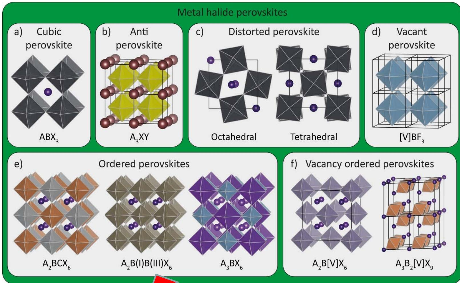
The **halide double perovskites**, or “elpasolites”, with formula  $A_2B'B''X_6$ . They can be conceptually derived from the standard  $ABX_3$  halide perovskite structure by replacing two  $B^{2+}$  cations with one monovalent ( $B'$ ) and one trivalent ( $B''$ ) cation;
