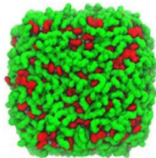
According to NMR, both carboxylic acids and amines are present and intermixed on the surface of double perovskite nanocrystals
