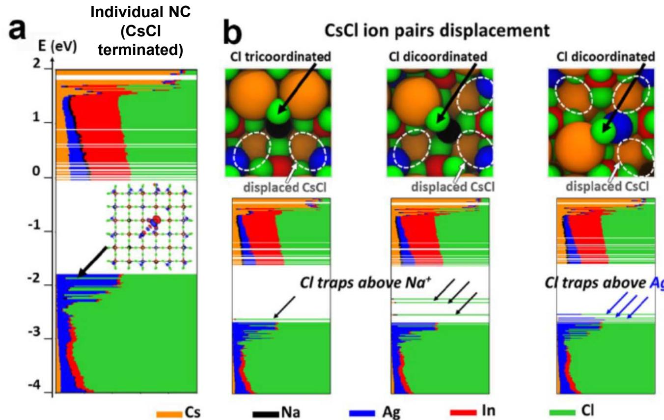
The displacement of CsCl ion pairs from the surface of the NCs simulates a partial decapping of the NCs
