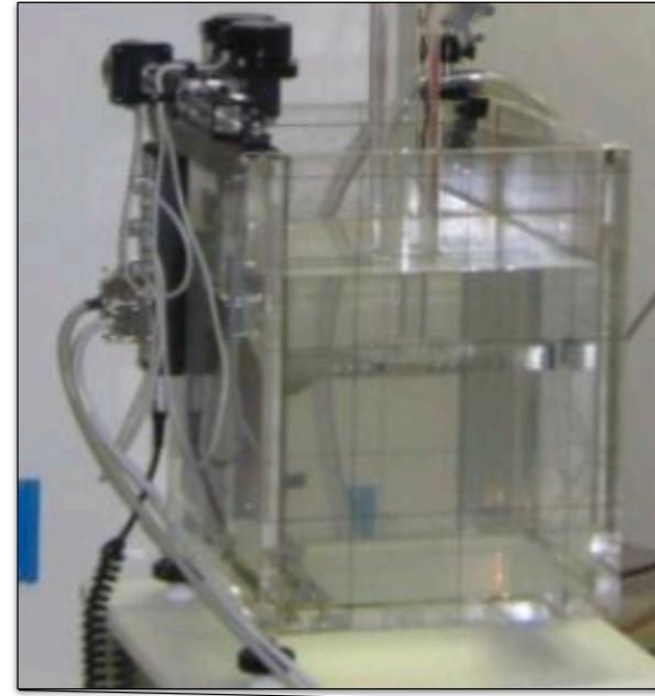
Measurements have been performed by SIT operators with a diode of 4 mm<sup>2</sup> placed inside a water tank.
