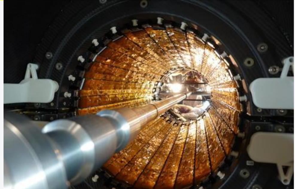
In the **ALICE experiment**, most of the detected particles by means of energy loss measurement like barions, mesons and nuclei are MIP's. PID is performed by the Inner Tracking System (ITS) and by the Time Projection Chamber (TPC).
