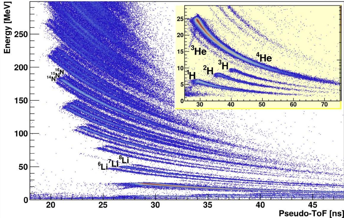
**ToF without a dedicated start detector** (working also for no pulsed beams).
