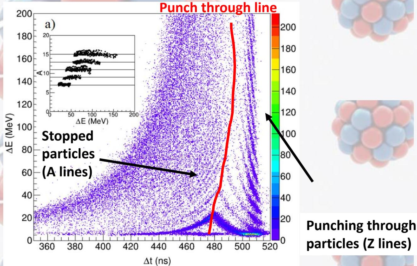
$\Delta A/A \sim 1/20$  with an energy threshold of 5 MeV/nucl
