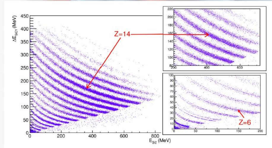
Pulse shape identification plot for particles stopped in the SiC (100  $\mu\text{m}$ )
