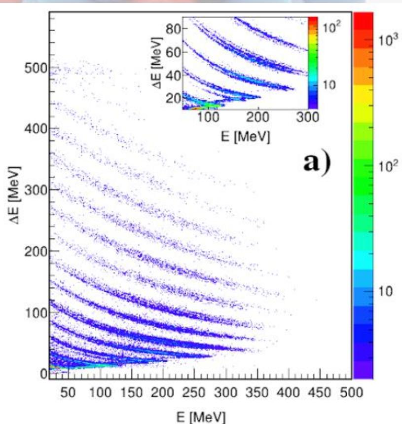
$\Delta E$ -E plot obtained using a telescope of the FARCOS array in the reactions  $^{124}\text{Xe}+^{64}\text{Zn}$ ,  $^{64}\text{Ni}$  at 20 MeV/nucleon.
