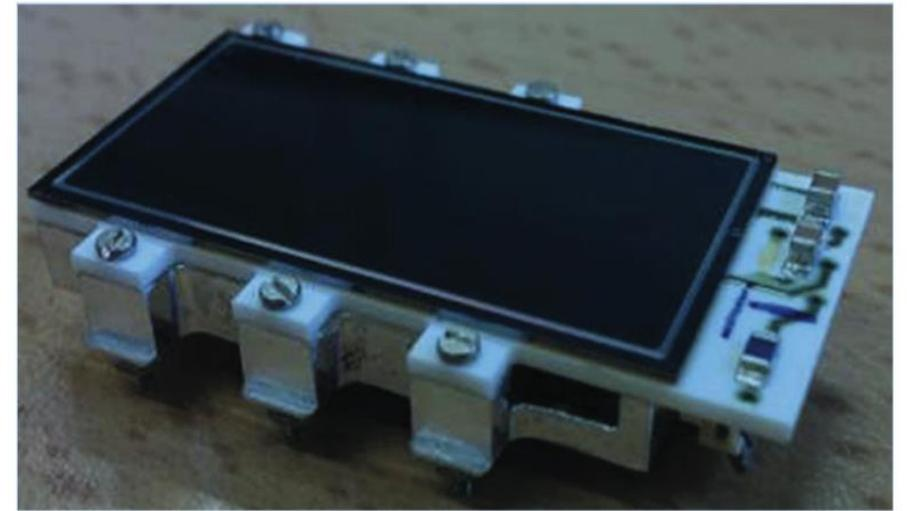
The SIDDHARTA-2 SDD array together with the readout electronics.
