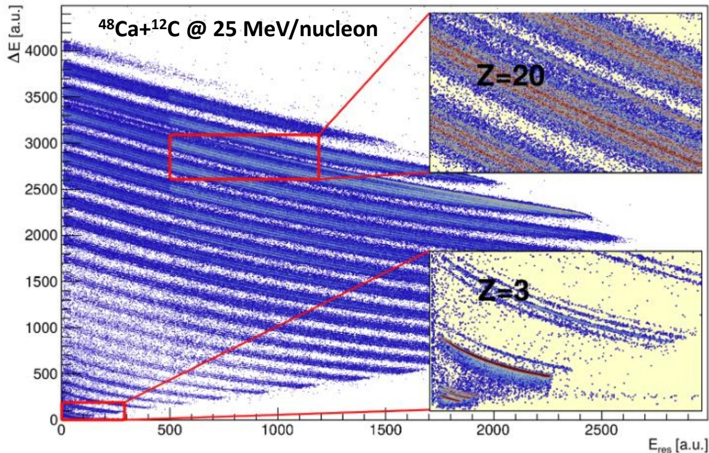
$\Delta E$ - $E$  correlation in a typical FAZIA telescope (first vs second silicon layer)
