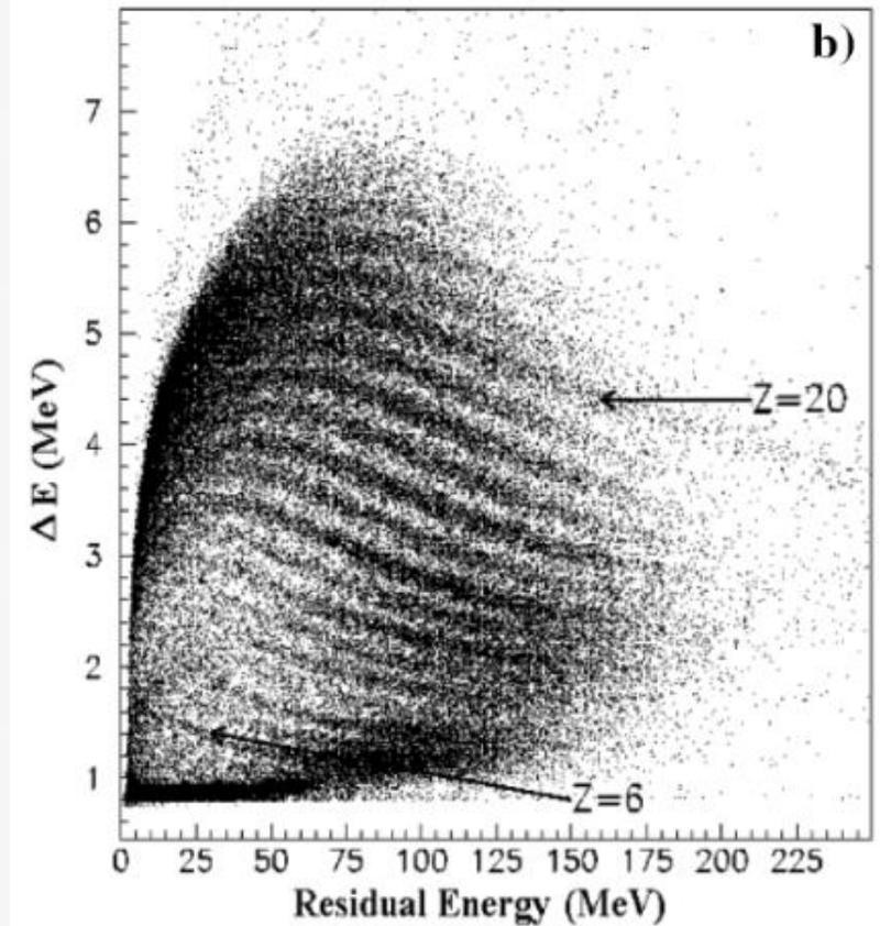
In nuclear astrophysics, beam energies and the energies of the emitted particles are often very low, so the energy loss in standard Si detectors may stop the impinging particles and no  $\Delta E$ -E spectra could be deduced
