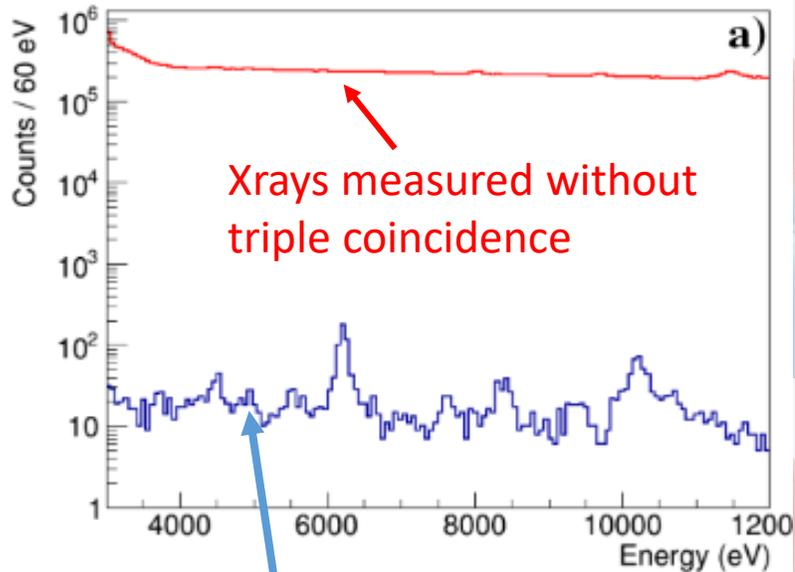
Triple coincidence between TOF (to measure K+K-) and SDD (to measure Xrays)=> very good background suppression
