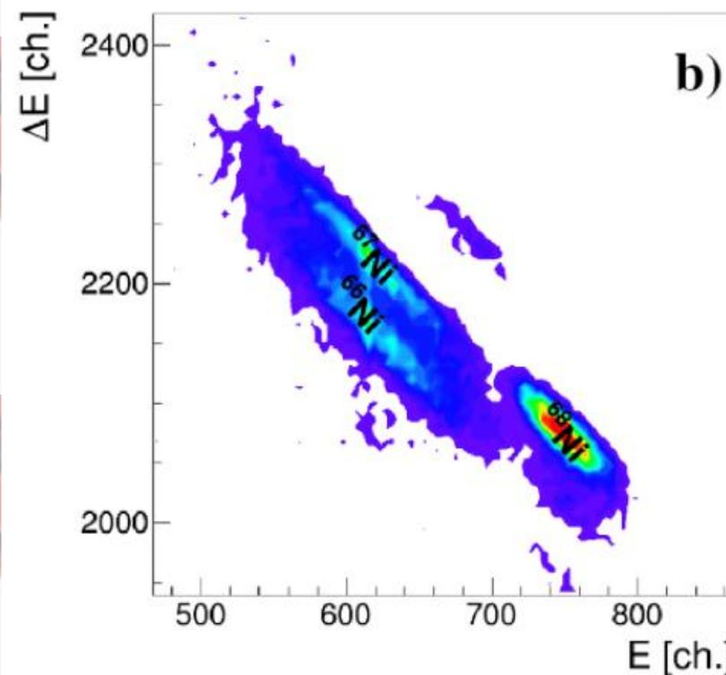
$\Delta E$ -E plot obtained in the reaction  $^{68}\text{Ni}+^{12}\text{C}$  at 28 MeV/nucleon. The  $\Delta E$ -E plot was obtained considering a strip of the 300 $\mu\text{m}$  stage and the corresponding strip of the 1500  $\mu\text{m}$  detector, for a FARCOS telescope
