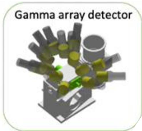
The  $\gamma$  array detector **GASTLY** has been developed and installed at CIRCE since 2018 to study nuclear reaction with charged particle in exit channel.
