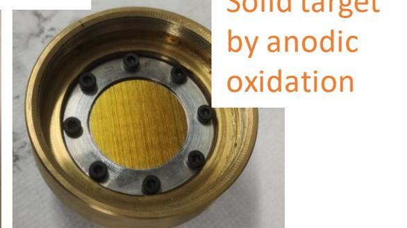
Solid target by anodic oxidation
