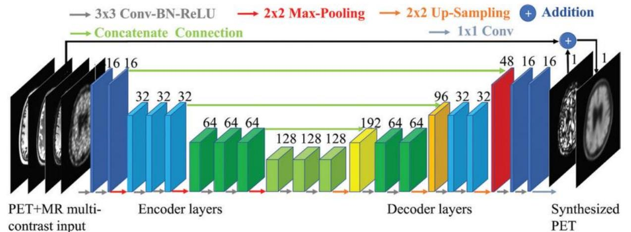
**Figure 1:** A schematic of the encoder-decoder convolutional neural network used in this work. The arrows denote computational operations and the tensors are denoted by boxes with the number of channels indicated above each box. Conv = convolution, BN = batch normalization, ReLU = rectified linear unit activation.
