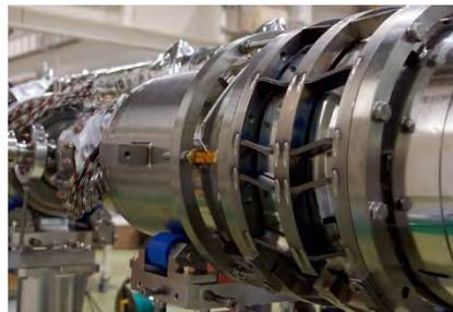
INFN Tuner for the ADS cryomodule at IPN-Orsay, **France**
