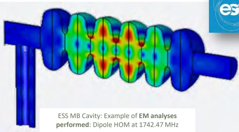
ESS MB Cavity: Example of EM analyses performed: Dipole HOM at 1742.47 MHz
