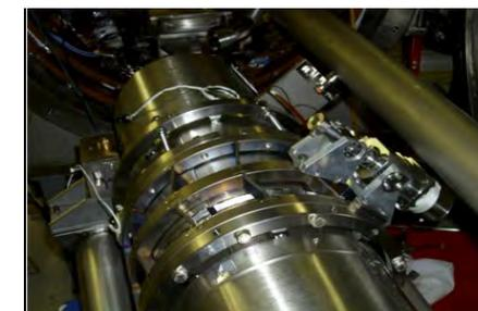
Piezoelectric actuators for fast tuning, E-XFEL, DESY
