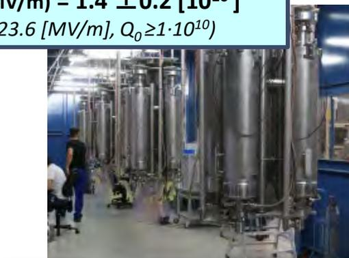
Cavities ready for the cold test
