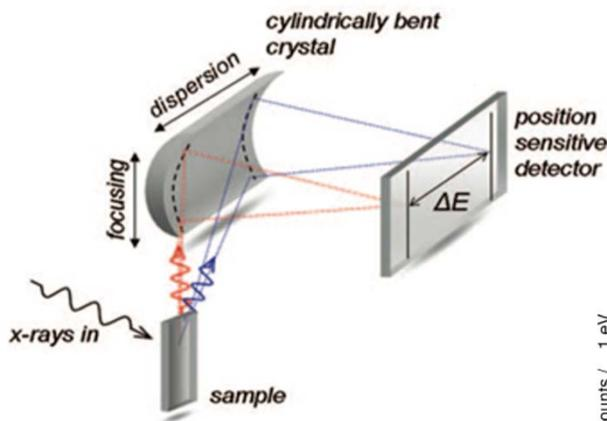
Von Hamos configuration to improve efficiency through vertical (sagittal) focusing properties of cylindrically bent crystals
