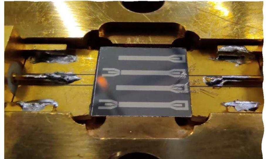
Prototype Devices fabricated at CNR-IFN with shadow mask evaporation technique
