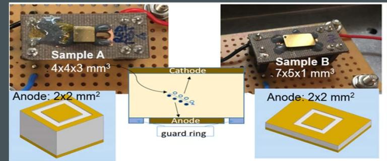
Cadmium(Zinc)Telluride detectors will be developed in the **STRONG2020-ASTRA**
