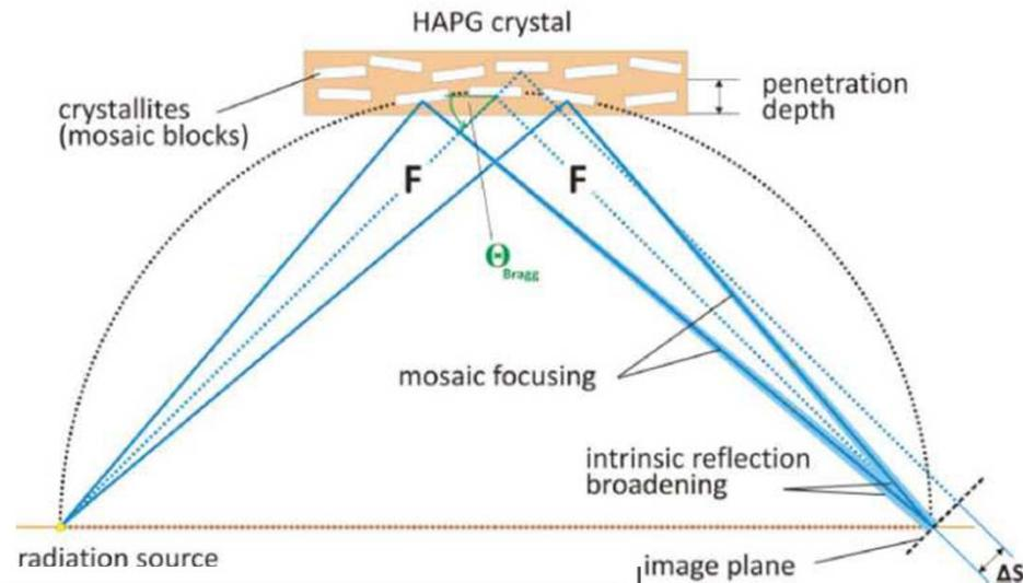
Mosaicity makes it possible that even for a fixed incidence angle on the crystal surface, an energetic distribution of photons can be reflected
