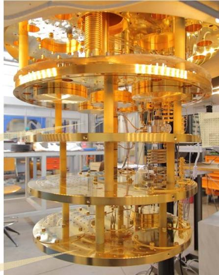
5 RF lines installed from 300 K to MixCh
