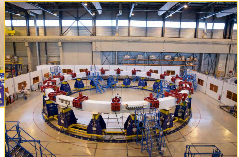
PF Coil #2 ready for resin impregnation, June 2020
