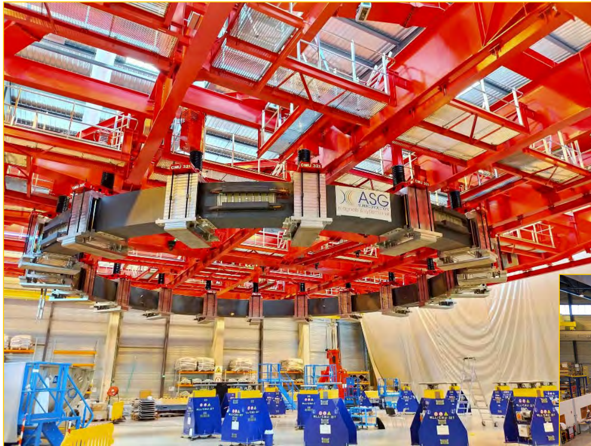
PF Coil #5 ready for cold testing, June 2020
