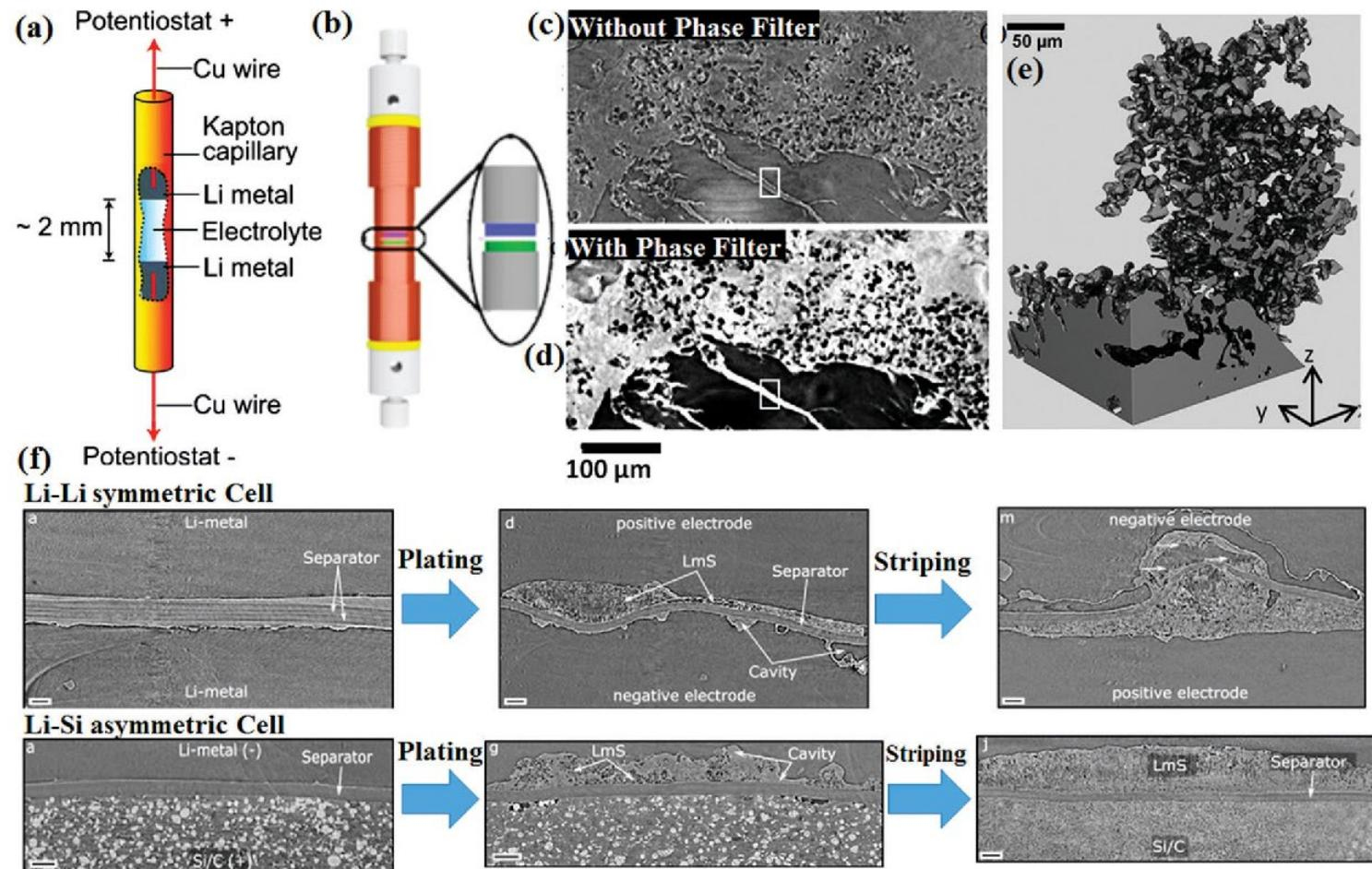
*In situ* X-ray tomography observation of lithium dendrites: (a) schematics of an *in situ* cell (Eastwood *et al.*)<sup>200</sup> Reproduced from ref. 200
