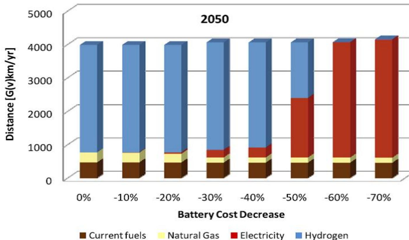
TIAM-ECN calculation of the distance travelled in 2050 by type of energy carrier for passenger cars in Europe under stringent climate policy and 100\$/bl oil prices with varying assumptions for the cost of batteries.
