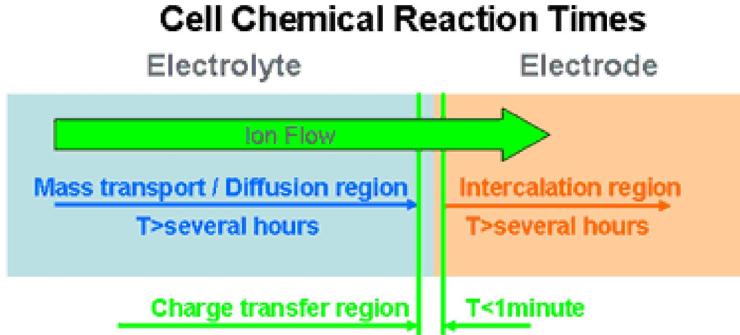
**Charge transfer / chemical conversion at the electrode surface (Short time constant)**
