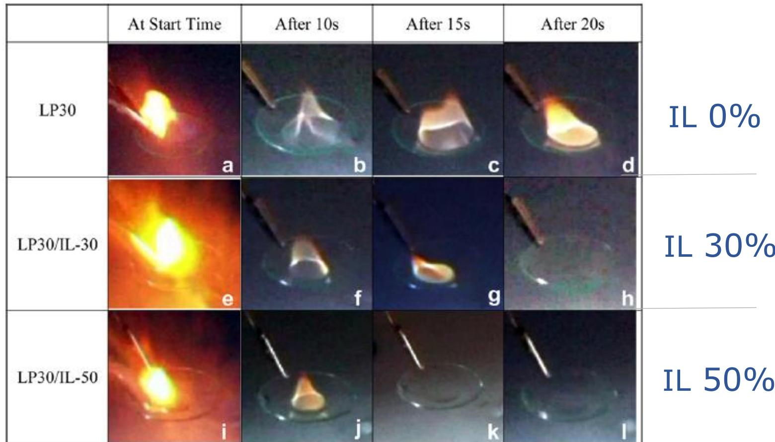
Pictures of the flammability performances of LP30 at starting time (a), after 10 s (b), after 15 s (c) and after 20 s (d); of LP30/ $\text{Py}_{14}\text{TFSI}$  70/30 wt/wt at starting time (e), after 10 s (f), after 15 s (g) and after 20 s (h); and of LP30/ $\text{Py}_{14}\text{TFSI}$  50/50 wt/wt at starting time (i), after 10 s (j), after 15 s (k) and after 20 s (l).
