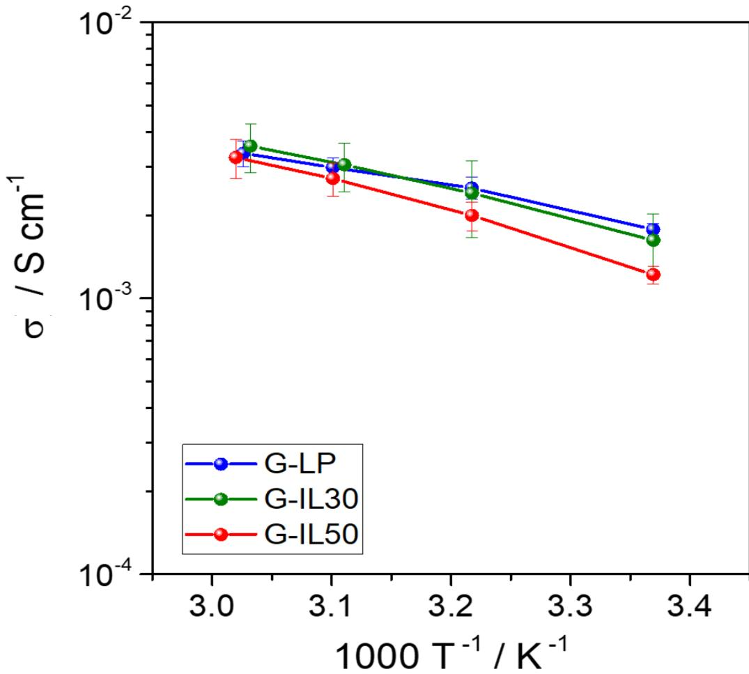
➤ All GPEs exhibit a room temperature ionic conductivity higher than  $10^{-3} \text{ S cm}^{-1}$ .
