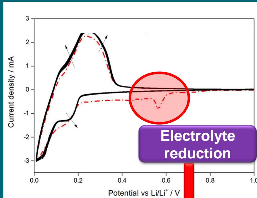
Anodic polarization (linear sweep voltammetry)
