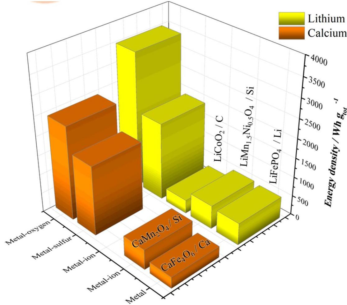
**CaMn<sub>2</sub>O<sub>4</sub>|Si** Ca-ion battery (CIB) can disclose a theoretical energy density of about 520 mWh g<sup>-1</sup>, overcoming the benchmark LiCoO<sub>2</sub>|C LIB (360 Wh kg<sup>-1</sup>) and approaching the theoretical figures of the LiMn<sub>1.5</sub>Ni<sub>0.5</sub>O<sub>4</sub>|Si and LiFePO<sub>4</sub>|Li formulations.
