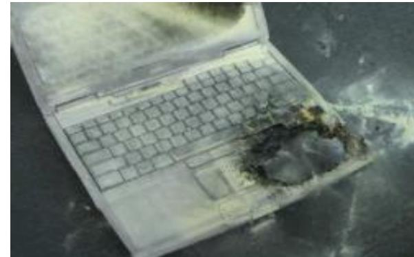
A Dell computer went on fire in a conference in Osaka in June 2006. Sony and Dell announced recall of Sony's lithium ion batteries packs (more than 4.5 million).
