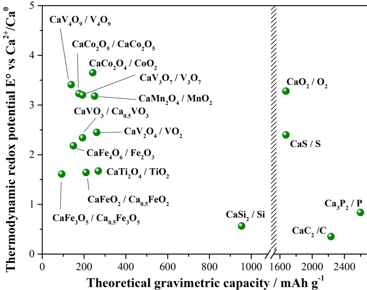
Even though calcium has an atomic weight 7 times larger than lithium, the specific capacities of the **oxides** vary in the  $100\text{-}250 \text{ mAh g}^{-1}$  range. Their capacity and thermodynamic potentials match the figures of lithium intercalation positive electrodes!
