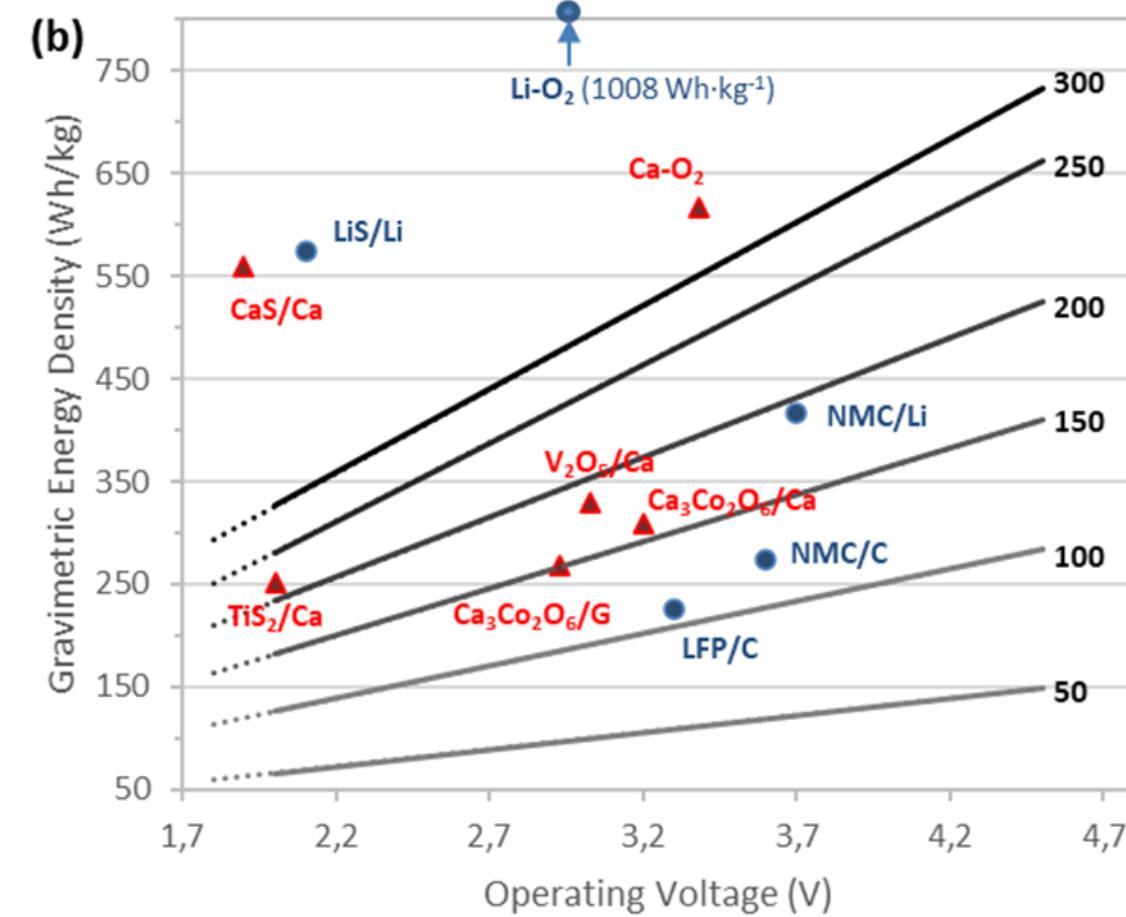
Volumetric (a) and gravimetric (b) energy densities for Li based batteries (blue circles) and Ca battery technologies (red triangles). The straight lines are calculated energy densities of hypothetical Ca metal batteries as a function of operation potential and cathode specific capacities (on the right of each line).
