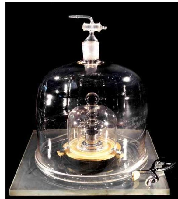
Shown: International Prototype of the Kilogram, kept at BIPM
