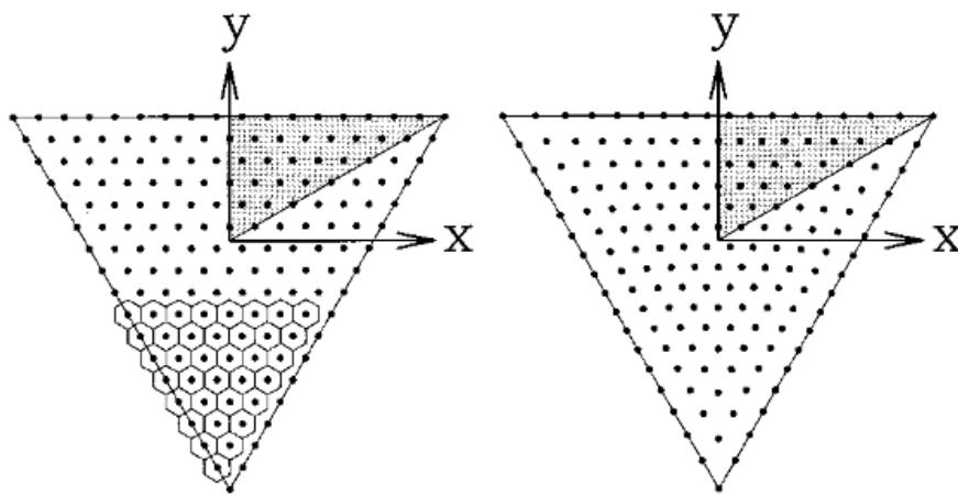
FIG. 2.—A regular triangular grid (*left*) is adjusted (*right*) to give all pixels the same area. As illustrated, the pixels have a hexagonal shape. A triangular icosahedron face can be symmetrically decomposed into six identical right triangles (one is shaded), and the area-equalization mapping is seen to respect this symmetry.
