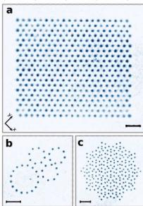
Whitlock group: Preparation of hundreds of microscopic atomic ensembles in optical tweezer arrays; NPJ quantum (2020)
