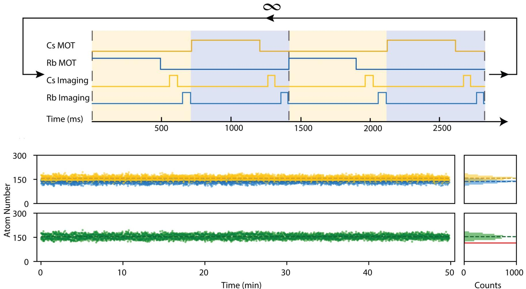
We can design experimental cycles where there are always atoms within the tweezer array available for measurements or computation
