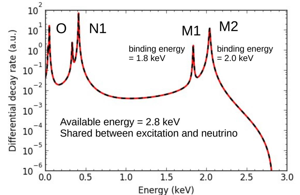
$$\frac{dW}{dE_C} = A(Q_{\text{EC}} - E_C)^2 \sqrt{1 - \frac{m_\nu^2}{(Q_{\text{EC}} - E_C)^2}} \sum_H B_H \varphi_H^2(0) \frac{\frac{\Gamma_H}{2\pi}}{(E_C - E_H)^2 + \frac{\Gamma_H^2}{4}}$$
