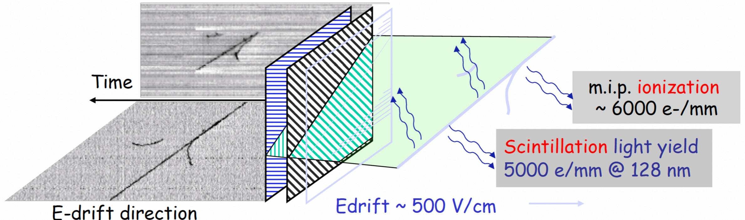
Drifting electrons are moving to transparent wire arrays oriented in different directions, where signals are recorded.
