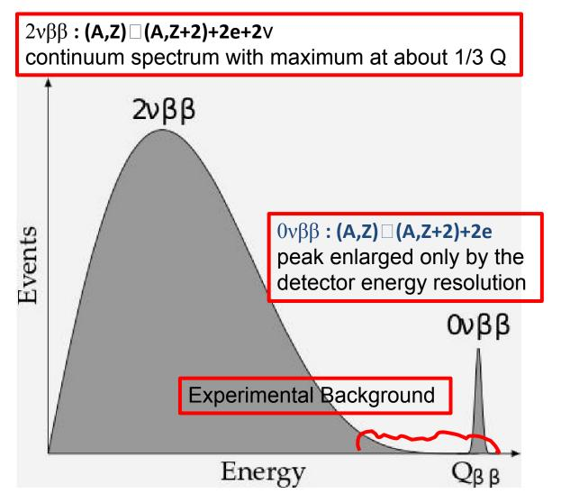
Experimentally a peak will be produced by the sum of the energy acquired by two electrons in the decay
